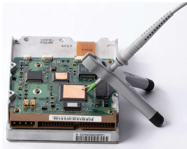
Figure 8. An IC cap adapter and ground blade with optional N2886A two-leg probe positioner offers an ideal hands-free solution for short circuit-proof probing of a fine-pitch IC. The N2877A deluxe accessory kit and N2878A fine-pitch accessory kit contain one N2886A two-leg probe positioner.
