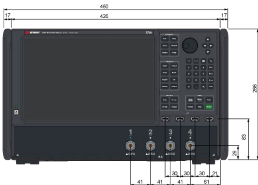
Dimensions (front view, E5080B with option 4M0/4N0/4M2/4N2 (2.4 mm connectors), in millimeters)
