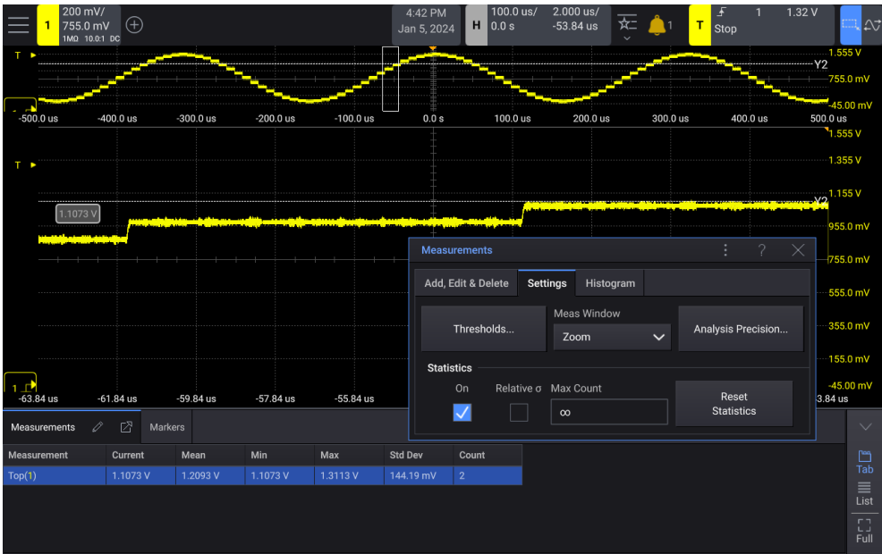
Figure 40 Isolating area for Top measurement
