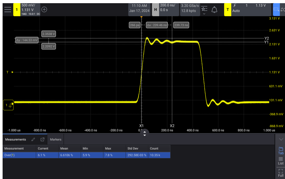
Figure 41 Automatic Overshoot measurement
