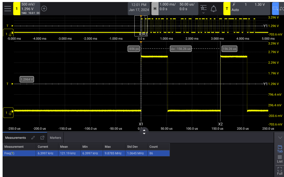
Figure 42 Isolating an event for Frequency measurement
