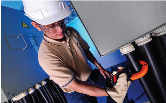
Figure 2. Large jaw clamp opening of 52mm / 2 inches
