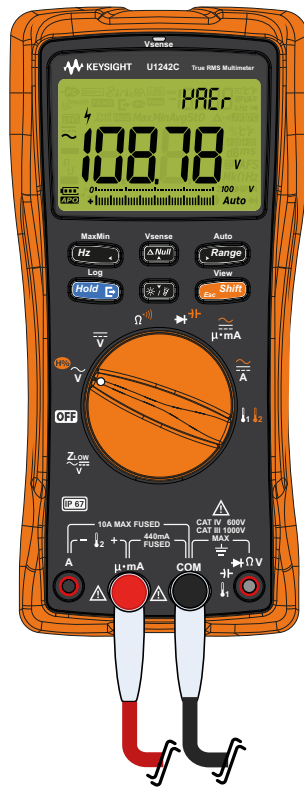
Figure 1-3 Example of \mu\text{AER} for wrong terminal input
