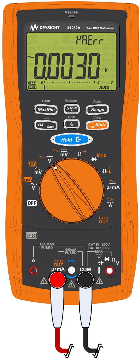
Figure 1-3 Example of \mu\text{AErr} for wrong terminal input
