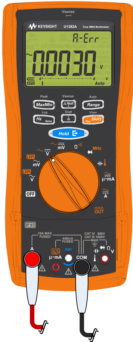
Figure 1-2 Example of A-Err for wrong terminal input
