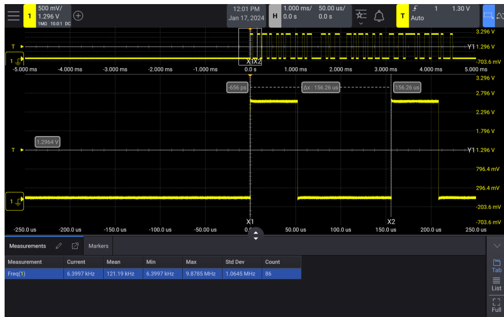
Figure 42 Isolating an event for Frequency measurement
