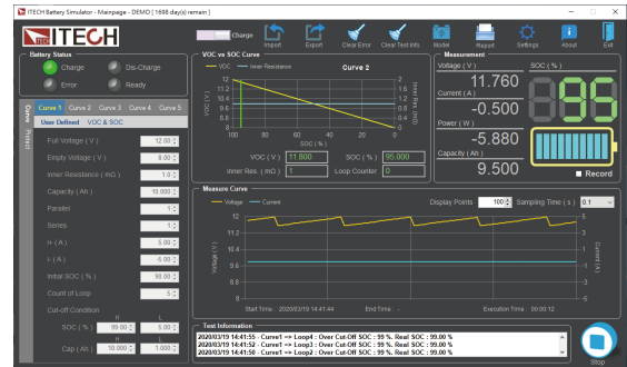
BSS2000 battery simulation software interface
