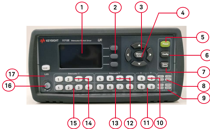
Figure 1-3 11713E front panel features
