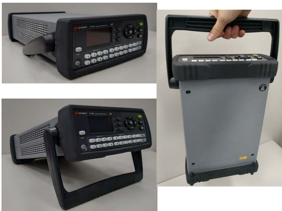
Figure 2-1 Handle positioning for bench operation
